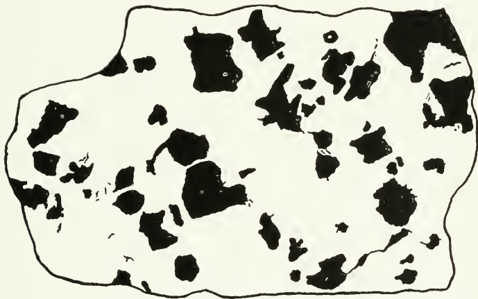
Fig. 62—"Spotted" diorite, actual size, Frood ore body, Sudbury area, Ontario. Black represents sulphides; white represents diorite. The sulphides replace or impregnate the rock.
